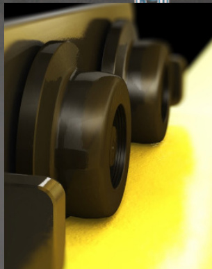
TROLLEY WHEEL WITH CAMBERED PROFILE
