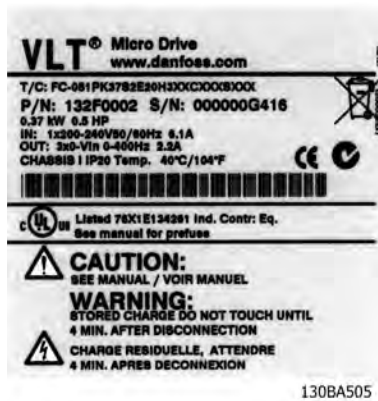
Illustration 2.1 This Example Shows the Nameplate Sticker
