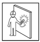
The zero-g safety function can prevent the uncontrolled output of commands in specific emergencies. The G sensor can detect if the transmitter receives a hard impact, dropped or thrown. These features can deactivate either the complete radio system or only the safety-relevant function relays. Alternately, a pre-defined output (e.g. crane horn) can be triggered. Please contact your dealer for special settings.
